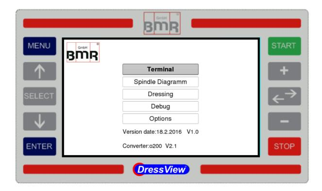
In the Main Menu all functions of the *DressView*®-system can be accessed. Moreover it shows the date and number of version, the type of converter being connected and it's number of firmware version.
