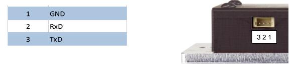
Attention, Interface is not galvanically isolated! X4.3 GND is connected with X2.2 OV.
