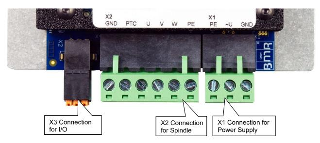
The PE connections of spindle and power supply can be connected at X2.
