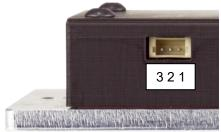
Attention, Interface is not galvanically isolated! X4.3 GND is connected with X2.2 OV.
